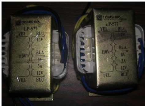
Figura 4.18 Transformadores 120Vac/24Vac- 3 Amp
