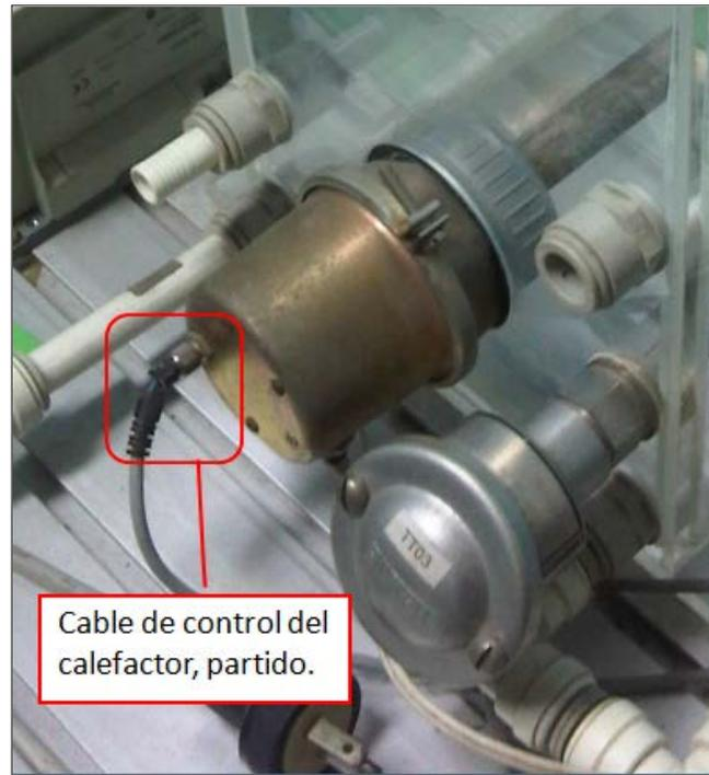
**Figura 4. 4 Cable del calefactor.**
