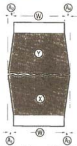
FIG. 7 Halves of Broken Charpy V-Notch Impact Specimen Illustrating the Measurement of Lateral Expansion, Dimensions A_1 , A_2 , A_3 , A_4 , and Original Width, Dimension W
