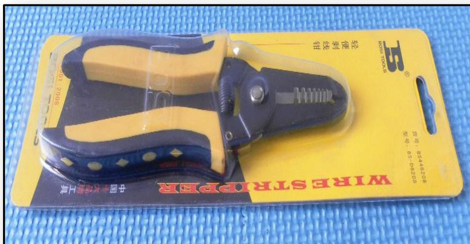
FIGURA 5.5 MULTIPROPÓSITO CORTA ALAMBRES BOSI
