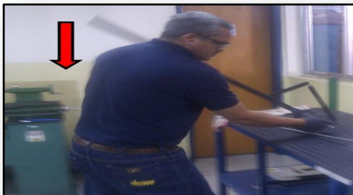
**FIGURA 5.14** CORTE DE MUESTRA CON CIZALLA MANUAL
