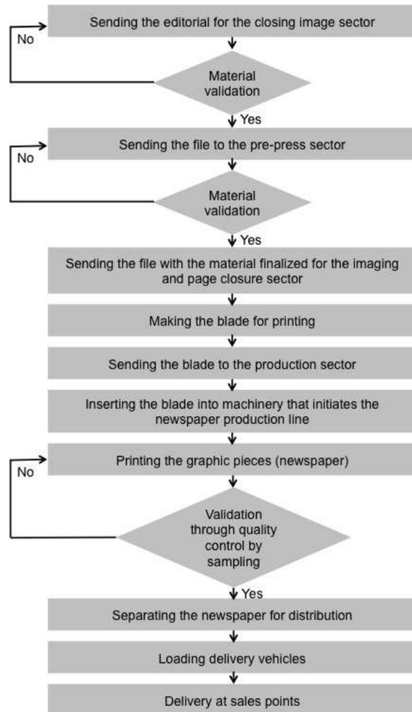
Figure 2: Production process flowchart of company A.
