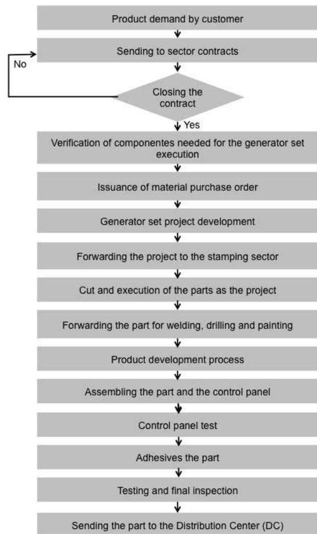
Figure 3: Production process flowchart of company B.
